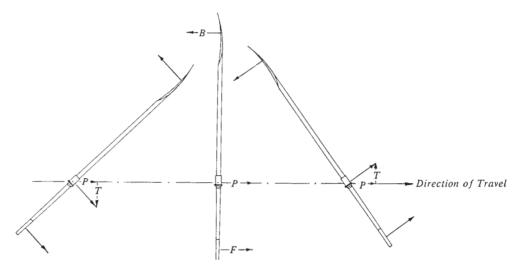
B – Pressure of blade against water. F – Force applied by athlete. P – Propulsive force. T – Turning force.
