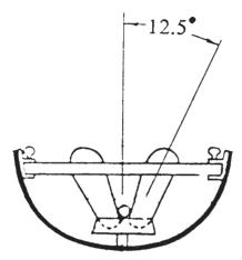
Figure 8: Opening angle of the foot stretcher
