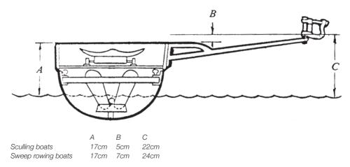
Figure 1: Immersed hull measurements
