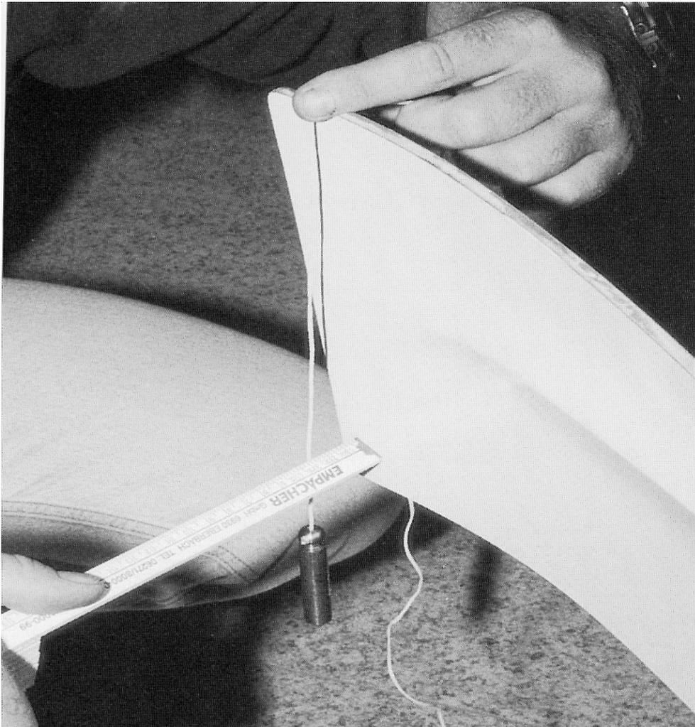
1. Place the oar perpendicular to the boat and hold it at a level comparable to its depth in the water.
