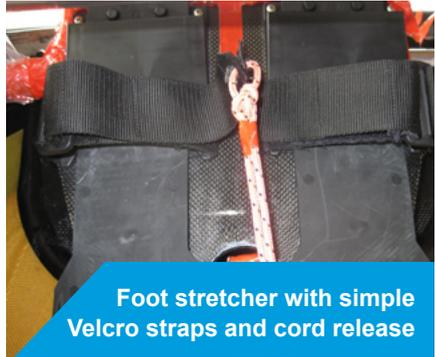
Foot stretcher with simple Velcro straps and cord release
